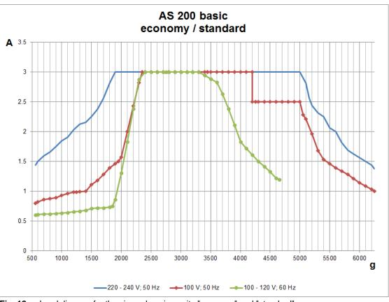
Fig. 12: Load diagram for the sieve clamping units "economy" and "standard"
