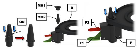
Fig. 6: Assembly of the clamping lid
