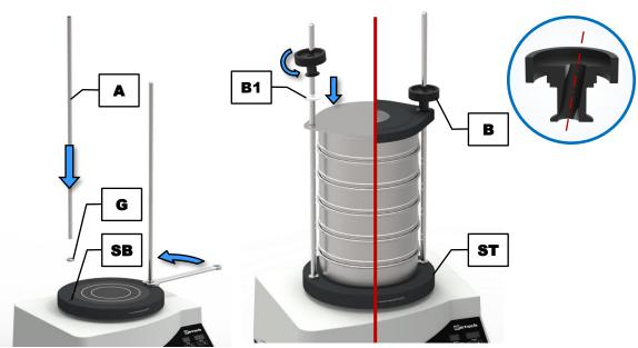
Fig. 5: Installation of the sieve clamping unit "economy" or "standard"
