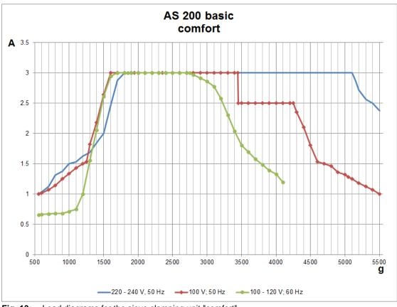
Fig. 13: Load diagrams for the sieve clamping unit "comfort"
