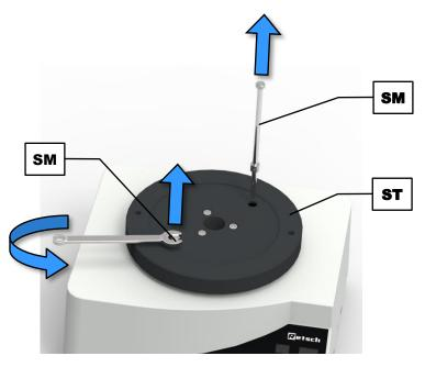
Fig. 2: Removing the transportation lock
