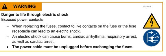
**NOTICE** Depending on the mains supply different fuses are used. The correct electrical protection is listed on the type plate  $(\mathbf{M})$ .
